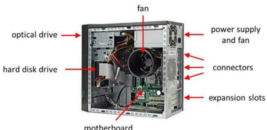
Figure 1.12 Central Processing Unit
